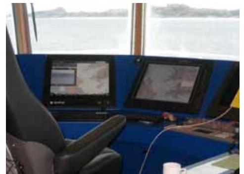
The information SECurus collects and integrates is displayed on an interactive touch screen on the bridge.
