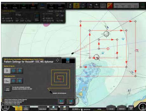
The SECurus' built-in search and rescue patterns can take wind, current and vessel speeds into account.
