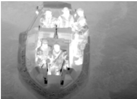
The FLIR MCT 3000 can detect small vessels at a distance of no less than 12 kilometers.
