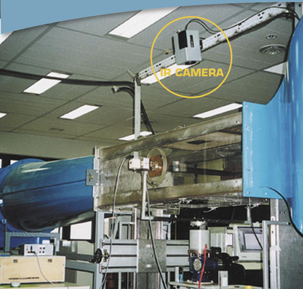
The wind tunnel with the ThermoCAM SC 3000
