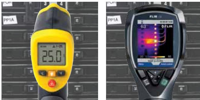
IR thermometer, temperature measurement in one spot FLIR i3, temperature in 3,600 spots
