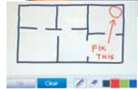
Multifunctional LCD touch screen allows sketching and marking directly on the screen.
