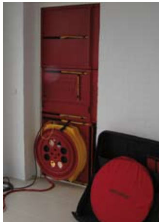
The blower door equipment is normally installed in the entrance door.
