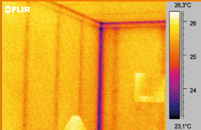
IR-image taken from the inside. The framework is visible, and so are the screws fitting the sheet covering to the framework. The corner is clearly colder, called a corner-effect, but there is nothing wrong here.
