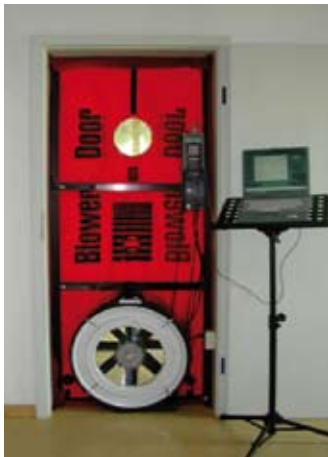
The blower door equipment is normally installed in the entrance door.
