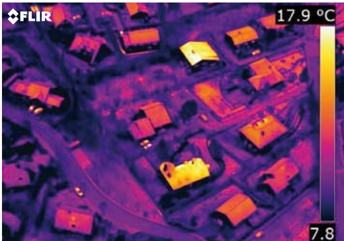
The buildings with yellow colored roofs show there is a moisture or insulation problem.
