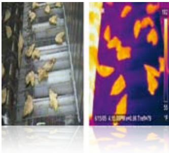
Figure 6. An IR temperature measurement and thermographic image are used to locate undercooked chicken tenders and stop the line so bad parts can be removed.
