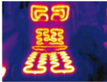
Figure 2. Production testing of car seat heater elements
