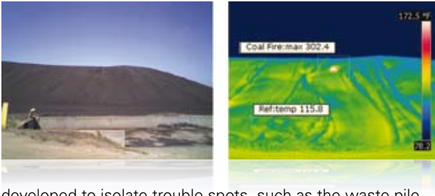
Figure 8. Visible light and IR images of a coal pile – the thermographic image clearly identifies a hot spot that is a fire about to erupt.
