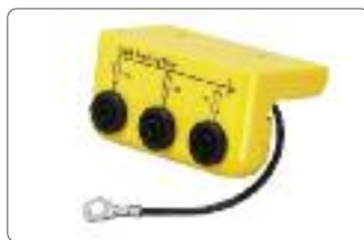
Description Order Code Bonding Panel with 3 4mm banana sockets, 1M \Omega resistor and 2m ground lead L-bracket type BLB-4-3
