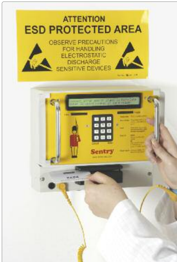
Sentry Grounding Facility Monitor
