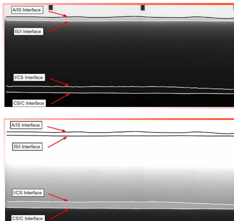
Fig. 3 Two montaged CCD images, using different contrast settings, of the studied cable joint combined with the binary interface image. The different layers in the cable are labelled for clarity
