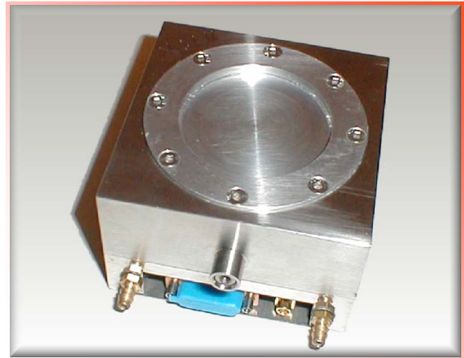
Fig. 1 The CCD camera head housing a CCD bonded to a scintillating fibre optic plate (SFO), supplied by Xcam Ltd.
