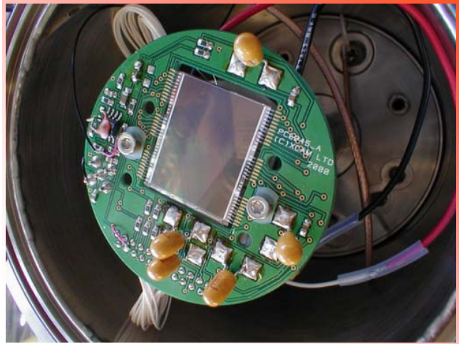
Fig. 1 A prototype custom CCD and headboard developed by Xcam Ltd for this work
