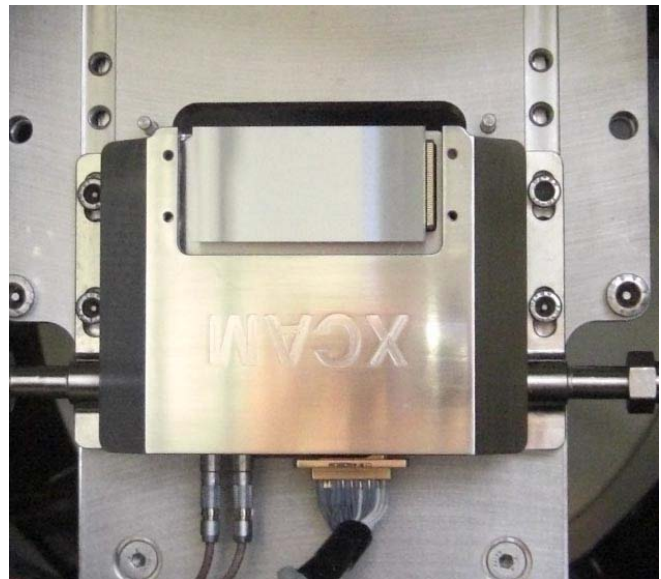
Fig 4: Single Unit Camera (below) in use inside vacuum chamber
