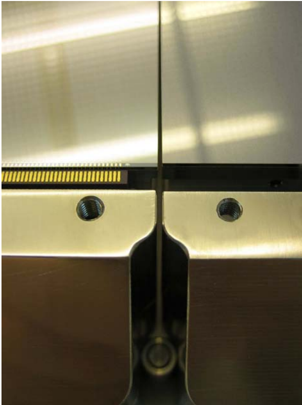
Fig 9: Showing Gauge Bush detail used to precisely set CCD separation down to 300 microns
