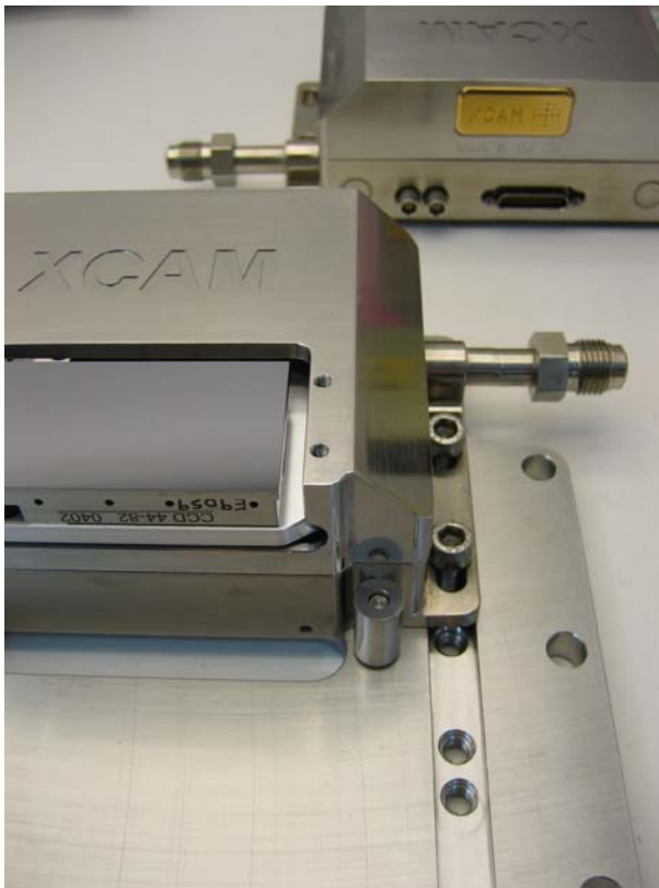
Fig 2: Xcam Single Unit on Base Plate in Foreground with Sensor Exposed to view, and (background) Alternative Orientation
