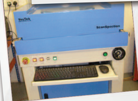
An in-line optical comparator has enhanced quality
