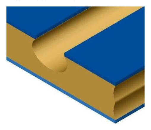
This characteristic can be very useful as half etch is used for fold lines and identification marks.
