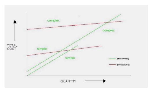
$Q = \underline{D - A}$  Pe - Ps Q = number of parts D = press tool cost A = phototool cost Pe = etched part cost
