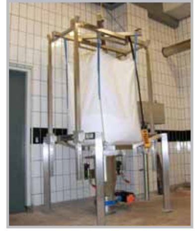
Stainless steel Model T1 with optional bag spout clamp.
