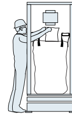
2. Bag spout and liner are opened up.
