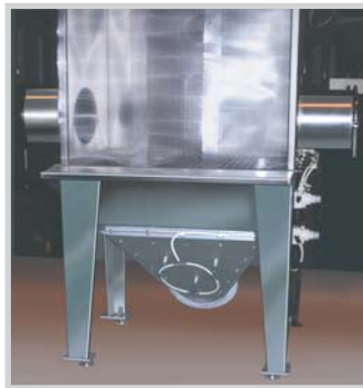
In sack emptying operations, a ▲ dust hood is often necessary. ▲ A sack compaction device may also be supplied.
