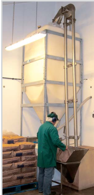
An AMC transferring flavoured coffee powder from a blender up to a packing machine.
