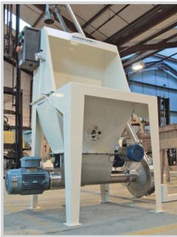
In sack emptying operations, a ▲ dust hood is often necessary. ▲ A sack compaction device may also be supplied.
