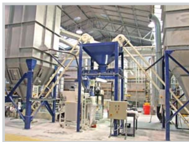
2 AMCs delivering tin oxide from process to packaging.
