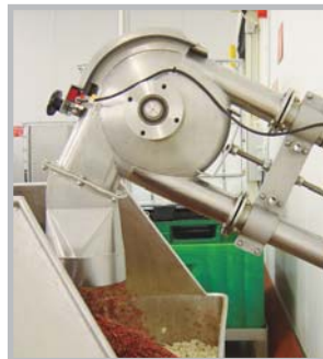
Interlocked inspection hatch in sprocket housing.
