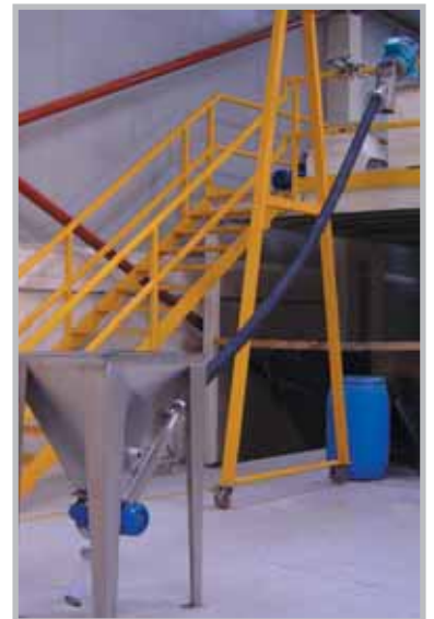
Our range of RHINOVEYOR Flexible Screw Conveyors are for very abrasive materials such as sand, cement and aggregates.
