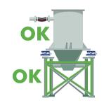
Take care to maintain a rigid supporting structure. Additional bracing may be required for safety and accuracy. Use flexible couplings to prevent lateral forces on the vessel
