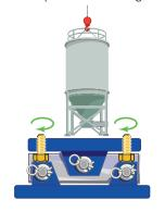
Use suitable jacking points. Lift or jack the weight off the load cell assemblies. Avoid excessive force. The dummy load cell must move freely.
