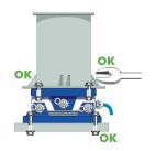
Check the load pins are secure, and the assemblies are bolted down before commissioning the weighing system.
