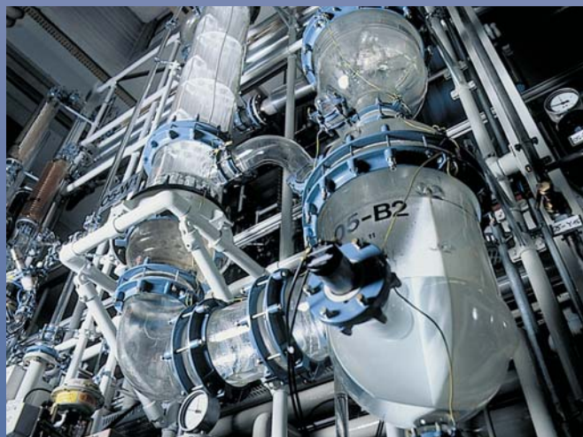
Large glass construction by Büchi, pilot plant and production scale. Options: SiC heat exchanger, gas scrubber, mixing vessel, etc.
