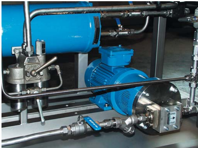
Lubrication oil circulation system.
