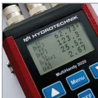
Two analogue, a frequency input and a calculated channel with min & max values
