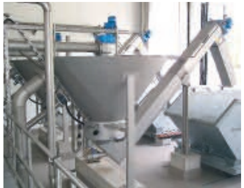
Innovative technology: COANDA Grit Washer RoSF 4
