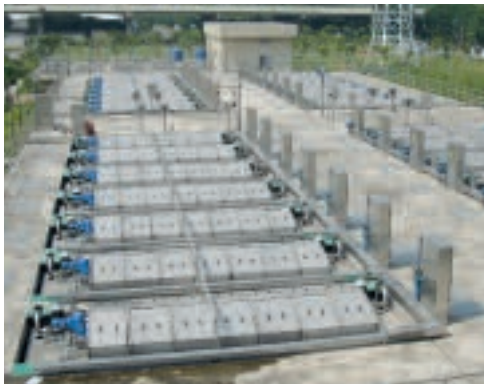
RoDisc® Rotary Mesh Screen with up to 30 discs in one unit
