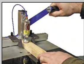
Swing-stops easily position material for repetitive holes
