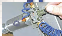
Each cylinder can be actuated individually or all at once with a master switch
