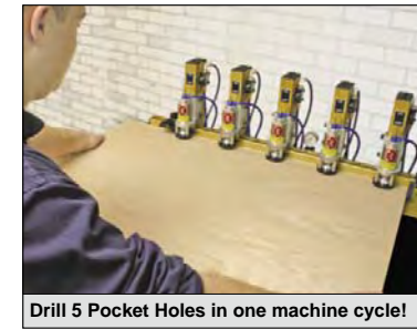
DK4100 - 4 Spindles, 8" on-center DK5100 - 5 Spindles, 6" on-center
