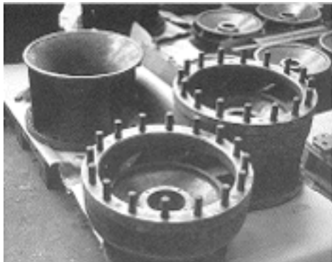
The badly worn internals of this Deepwell Multistage Pump were rebuilt and coated with Ceramic Metal giving extended life.
