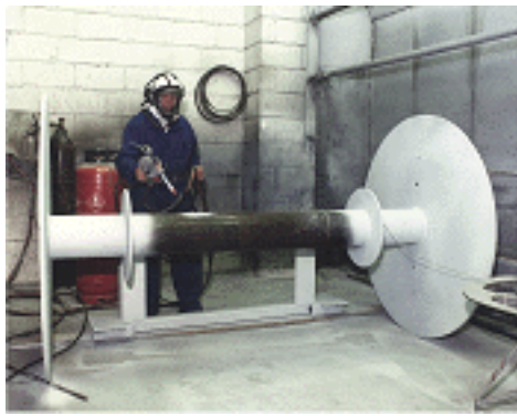
Metal sprayed coatings being applied to winch components for use in corrosive salt-water environment
