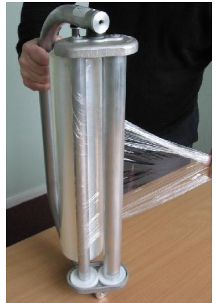
Thread under second roller
