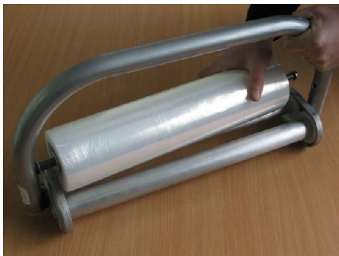
Compress spring by pushing roll and holder
