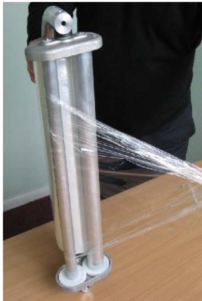
Wrap around first roller
