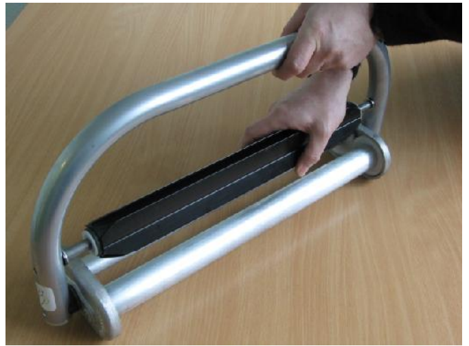
Compress the spring on the roll holder
