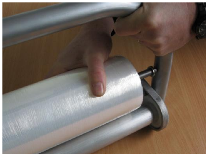
Insert opposite end of holder in to location point
