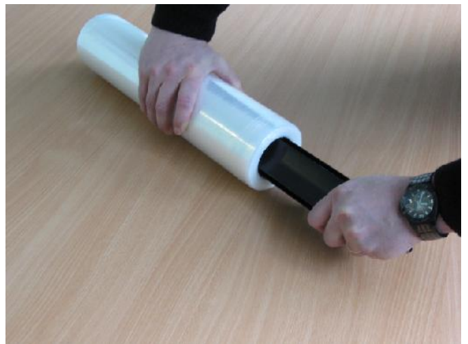
Push roll holder in to roll
