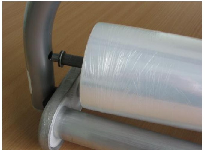
Locate roll holder in to location point
