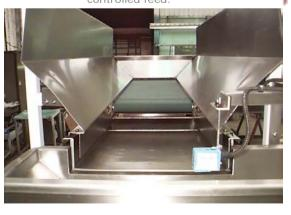
This twin bowl feeder & twin linear track feeder is supplying lids to a packaging line for confectionery products.
