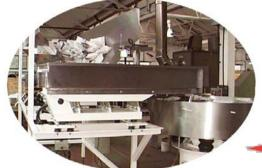
This system shows a linear feeder as part of a system incorporating a store-belt conveyor, and low frequency bowl feeder.
