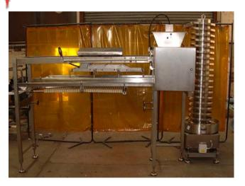
This unit is used to handle sugar coated jelly sweets. The section of wedge wire screen deck removes any sugar dust from the sweets. The feeder gives a controlled feed to the next part of the manufacturing process.
