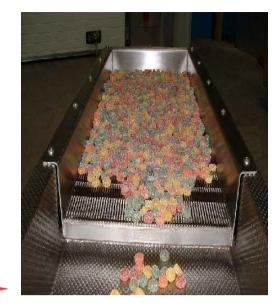
This unit was designed to elevate and feed toppings for confectionery. It transfers onto an electromagnetic prefeeder, and then onto a cascade sprinkle feeder to evenly spread the toppings onto the sweets below.
