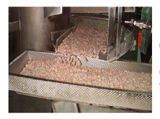
This picture shows a spiral lowerater / glazer. It transfers onto an electromagnetic linear feeder, and then on to automatic freezing and packing machine.
