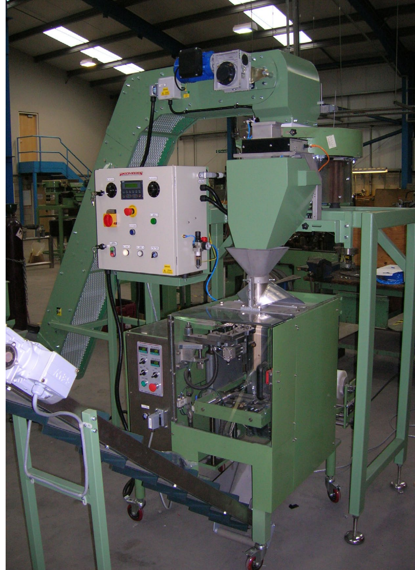
Right: Flighted belt elevator feeding counting & bagging machine.
