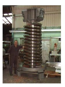
Low frequency vibratory spiral elevator driven by two vibratory motors mounted at the top of the unit. This unit is lifting coated snack foods to a packaging line.
