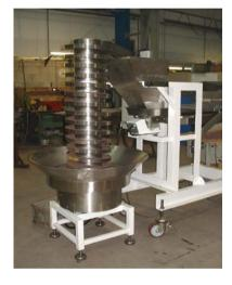
Twin motor driven, low frequency spiral elevator elevates plastic pellets into a receiving hopper. This allows the product to cool down between two manufacturing processes, whilst taking up only a small area of the limited manufacturing space available.
