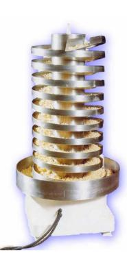
High frequency electromagnetic spiral elevator elevates chocolate shavings into receiving hopper. This is the pre-feed for a special system used to sprinkle the shavings onto cakes passing under a Vibratory spreader
