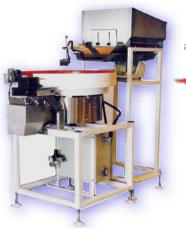
Podmores bowl feeders are available in a variety of materials to meet food, pharmaceutical, and industrial applications. This unit is feeding and counting surgical monolet needles into a pack sitting on a Vibratory consolidating unit.
