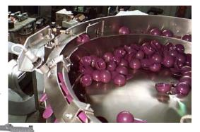
Here, a bowl feeder is being used to feed parts onto a linear track feeder. The parts accumulate in 6's at the end of the track where a pick and place unit moves them to the next manufacturing process.
