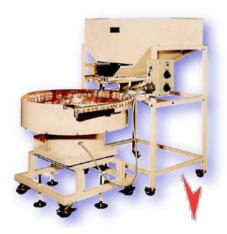
Plastic spice containers are fed from a bulk storage hopper into bowl feeder, which then feeds an automatic filling line.
