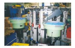
Two of four Bowl feeders supplying plastic components to a robotic assembly machine. The system assembles plastic roller bearings.
