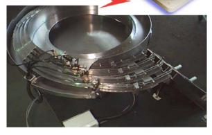
This bowl feeder is tooled with four tracks to allow the product to be split into four lanes before passing to the next manufacturing
