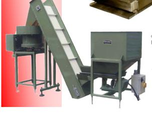
This flighted – belt elevator is being fed by an Electro magnetic Vibratory feeder, loaded via a bulk storage hopper. The system is used to provide a bulk and controlled feed to the bowl feeder.
