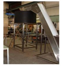
Here a corrugated walled sidewall belt elevator is lifting container caps into a high – level bowl feeder fitted with a "sound enclosure". The caps are fed from the bowl via a horizontal track feeder into the feed chute of an automatic cap placing and closing machine.
