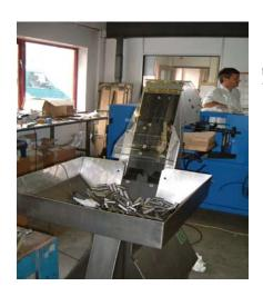
The Pneumatic step feeder shown here is used to elevate a range of steel tubes between 15-52mm diameter and 30 – 60mm long. They are loaded into an automatic
