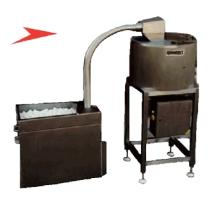
Podmores Cap Blowing Elevator lifts the caps from a bulk store hopper into the bowl feeder.
