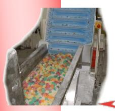
This Corrugated walled, flighted – belt elevator unit is taking jelly sweets from a store-belt conveyor and Vibratory cross – feeder. The unit discharges into a high level cross - head feeder and ultimately a multi head weigher.
