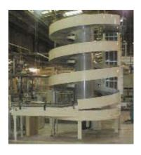
This plastic slat belt elevator / lowerator. Constructed from 304-grade stainless steel, with height and belt width options to suit your needs. Ideal for elevating within confined production / packaging spaces.
