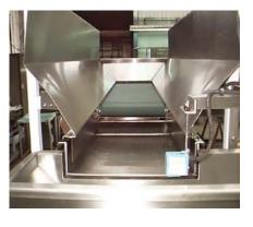
When a Bulk supply of product is required in a specific production run, a Store Conveyor can be used to supply both the required volume of storage and the required controlled feed in one item of equipment.
